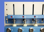
Figure 10. Three coin cell batteries being cycled
