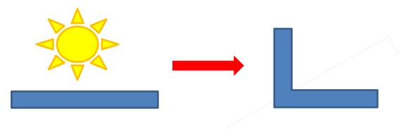
Simple actuator: the light causes the piece of plastic (blue) to bend
